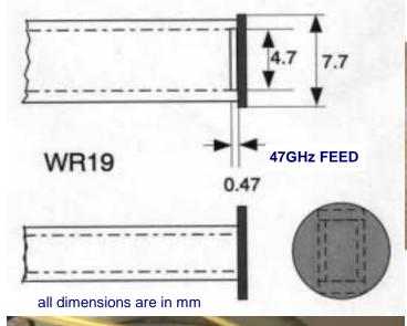
connector or .141 semirigid cable. 1,8mm of the teflon dielectric extends into waveguide. Length of pin above dielectric is 7,6mm. M3 tuning screw is diametrically opposite probe and is adjustable. 5760 MHz probe is 15,2 - 17,8mm in length and can be made from tubing 1,8 - 2,5mm in diameter. Tuning of both frequencies can be accomplished by tuning either probe length. Isolation:
