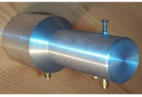
10368 MHz signal@ 5760 MHz port = -19dB 5760 MHz signal @ 10368 MHz port = -45dBReturn loss >23dB at both ports
